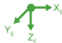
Earth-Fixed (Inertial) Coordinate System (Z-Down)
